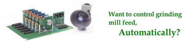
The *MillMinder* Audio Signal Converter listens to the sound levels generated by the impact inside the grinding mill and provides the operator with an output signal which allows automatic material feed control to the mill.
