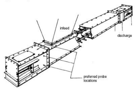
The Probe is mounted to monitor the T flight of the drag conveyor. The Probe should be mounted at the point of minimal vertical deflection, so as to avoid double pulsing, and where experience shows breakage occurs more often.
