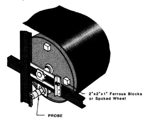
The preferred method for monitoring a belt conveyor is to mount  $2^{\circ} \times 2^{\circ} \times 1^{\circ}$  (50mm x 50mm x 25mm) ferrous blocks on the driver pulley. The blocks must be equally spaced as to assure a uniform pulse rate.
